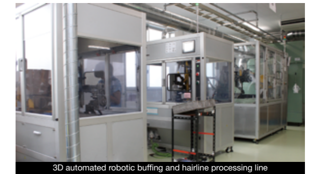
3D automated robotic buffing and hairline processing line
